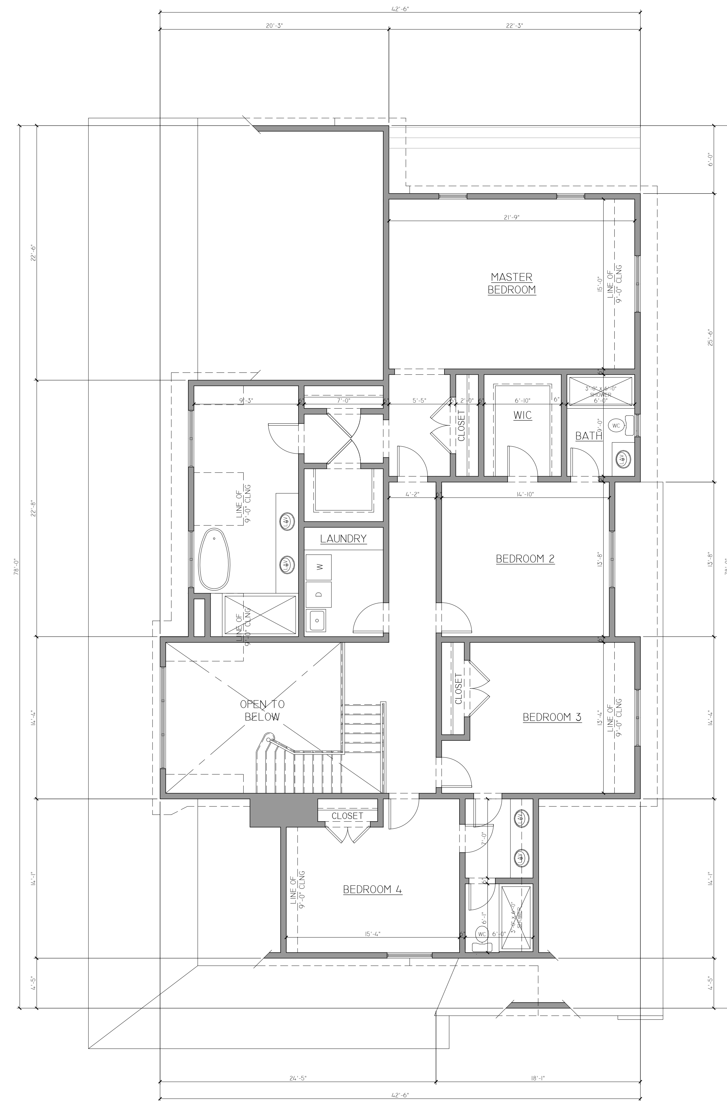
PROPOSED SECOND FLOOR PLAN SCALE -- 3/16"=1'-0" ARCHITECTURAL SECOND FLR LIVING AREA : 1,913 SF GROSS SECOND FLR BUILDING AREA (PER ORDINANCE) : 1,913 SF
