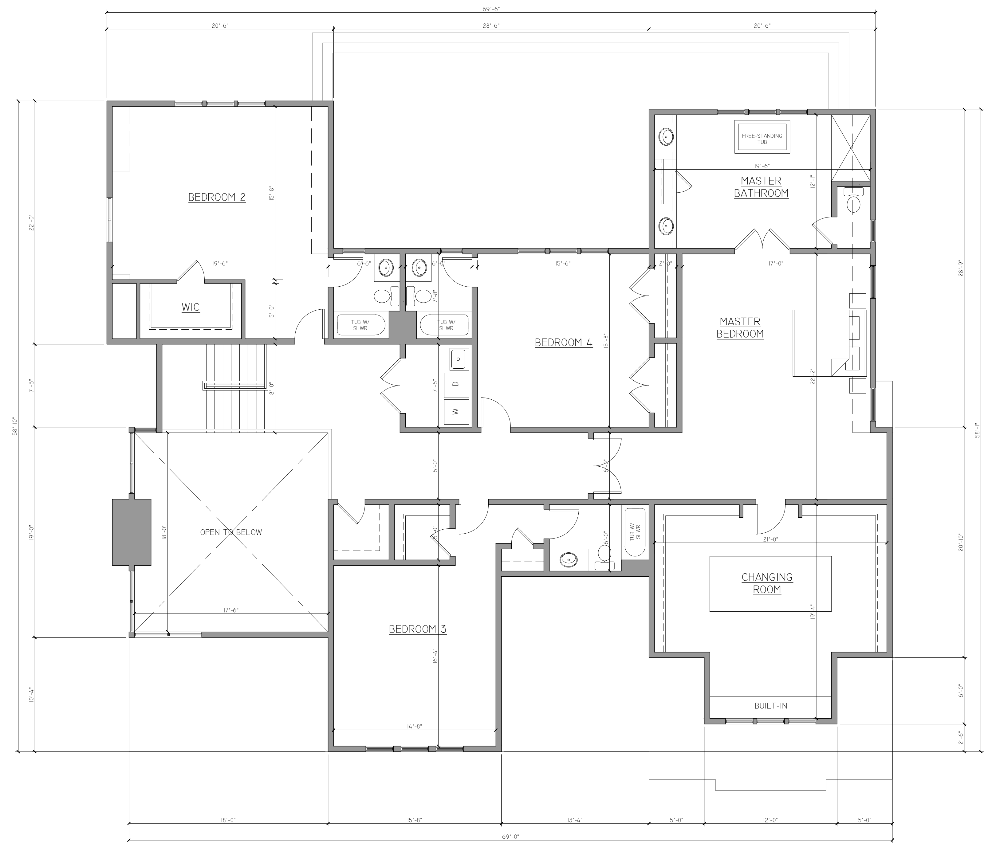
PROPOSED SECOND FLOOR PLAN SCALE -- 3/16"=1'-0" ARCHITECTURAL SECOND FLR LIVING AREA : 2,721 SF GROSS SECOND FLR BUILDING AREA (PER ORDINANCE) : 2,721 SF
