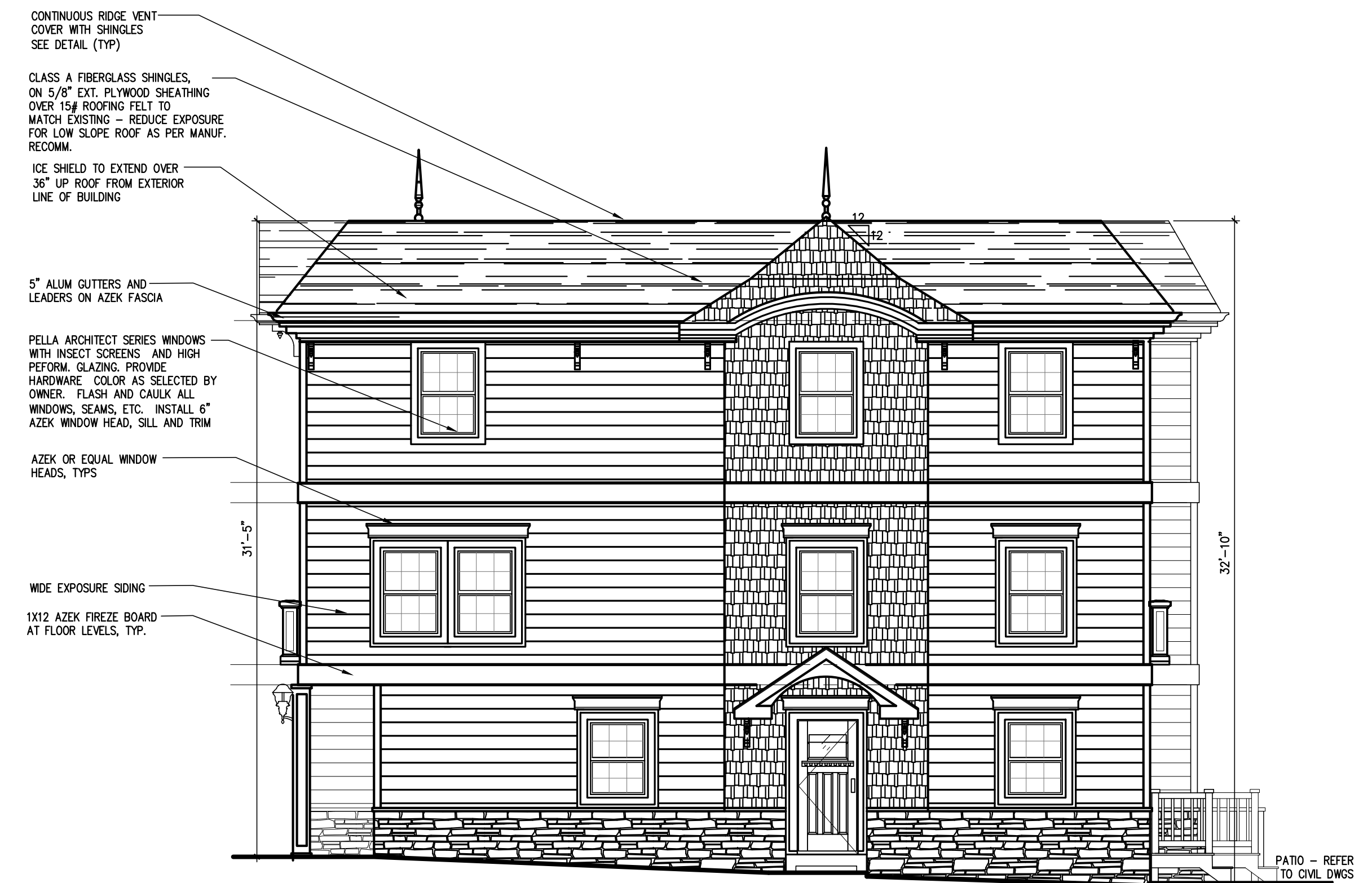
2 PROPOSED RIGHT SIDE ELEVATION (PARK AVENUE) SCALE: 3/16" = 1'-0"
